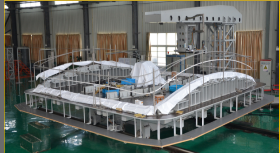
Correction coil at ASIPP in Hefei, China.
