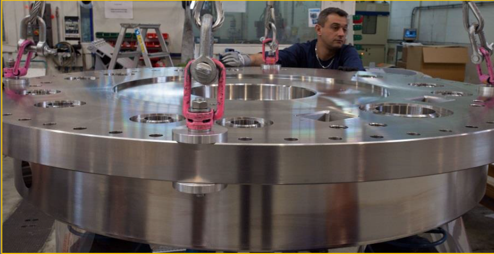
8-tonne machined flange of the first Torus Cryo-pump
