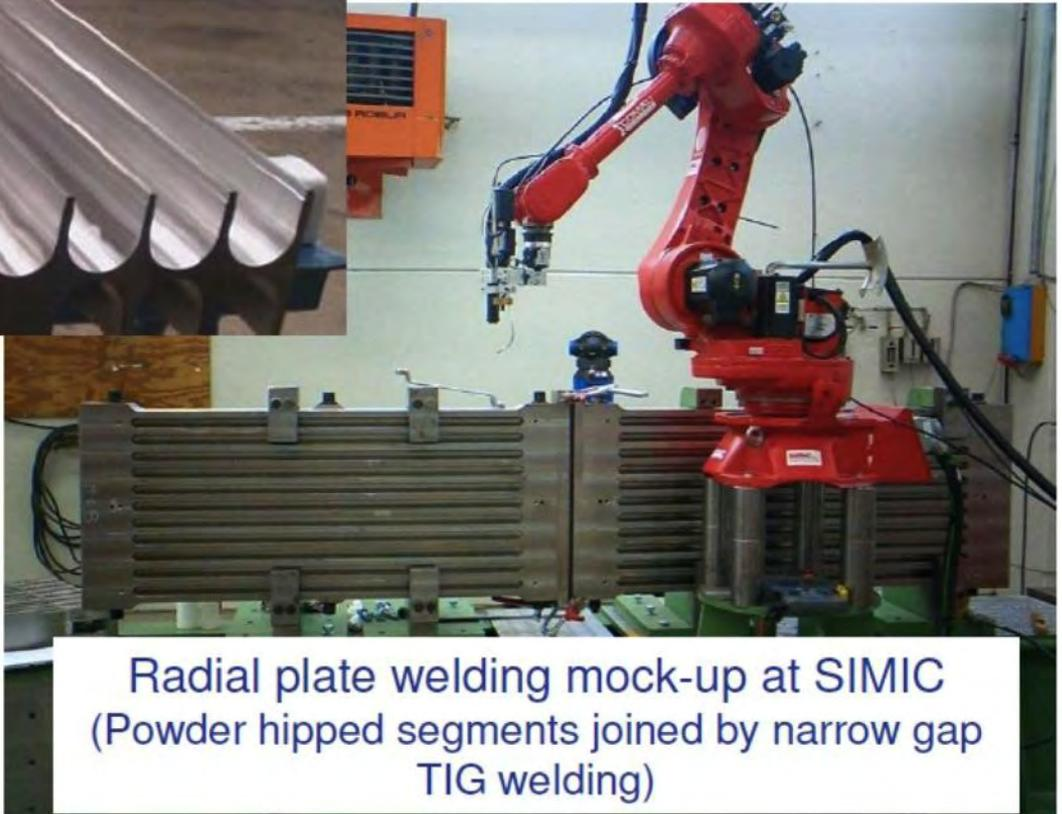
Radial plate welding mock-up at SIMIC
