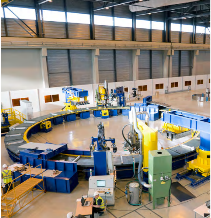
Installation of winding tooling, Poloidal Field coils facility, December 2015
