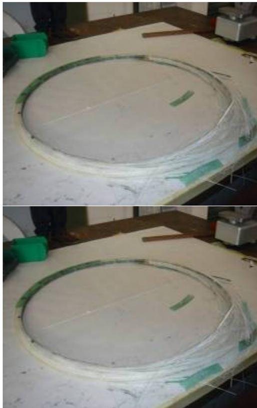
Figure 18 - Pre-compression ring mock-up after rupture
