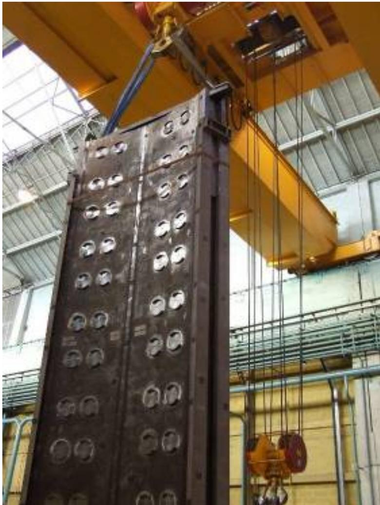
Figure 20 - Electron Beam Welded Sector Mock-up
