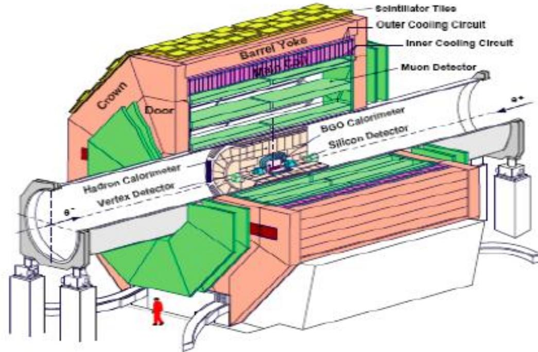
Only the muon detectors, the magnet and the scintillator tiles were used in the LEP (*L3+C Collaboration*) solar flare experiment of July 14, 2000.
