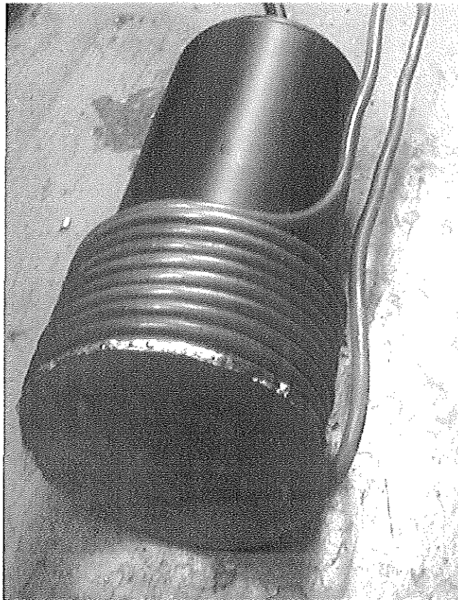
Fig. 11. The \gamma -detector shielded from thermal radiation by water-cooling.
