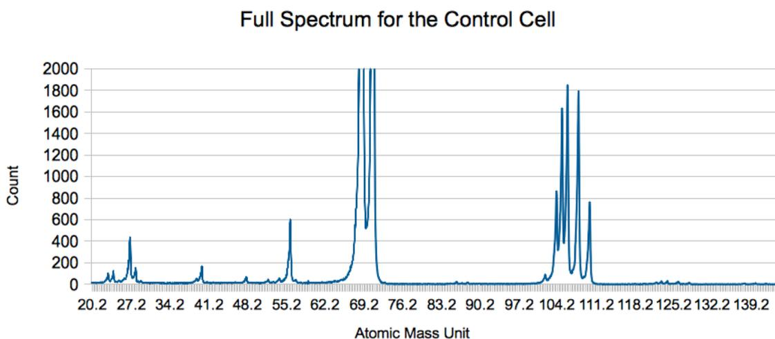
*Figure 25: SIMS Spectrum of the original palladium. The main peaks at the center are the gallium source. On the left the palladium shows its 6 isotopes. Are also present Fe, Al and small amounts of Ti and Mg.*
