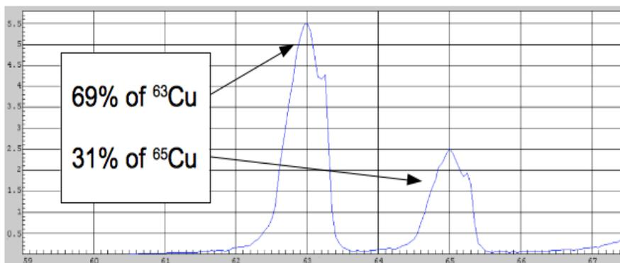
Figure 20: SIMS analysis of a copper dot. The amount of Cu(63) is 69% and the Cu(65) is 31%.
