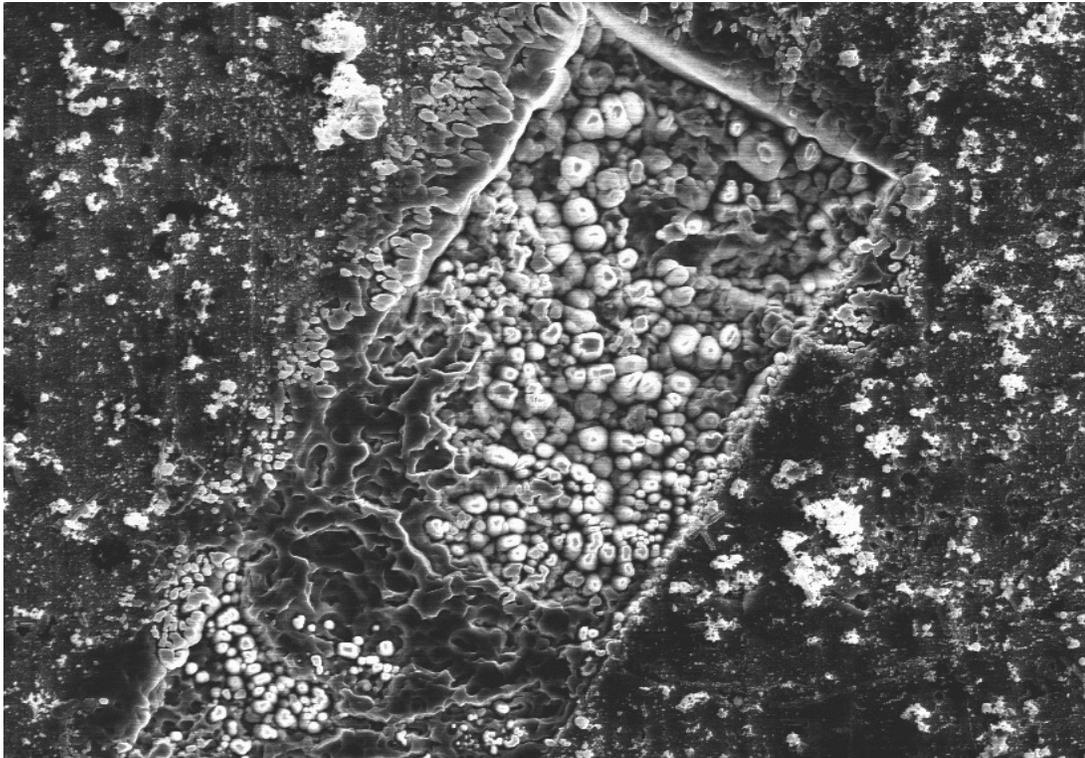
*Figure 22: SEM picture of a milling pattern made with high energy ion beam. The pattern is 50  $\mu\text{m}$  in width.*
