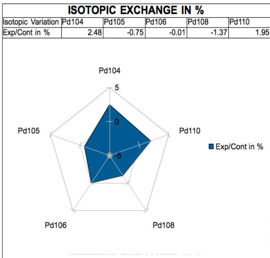
*Figure 31: Graph showing the calculated isotopic exchange of Pd loaded on April 2011. This shows for each isotope the percentage exchanged between the natural abundance and the corrected value of given by the calculation.*
