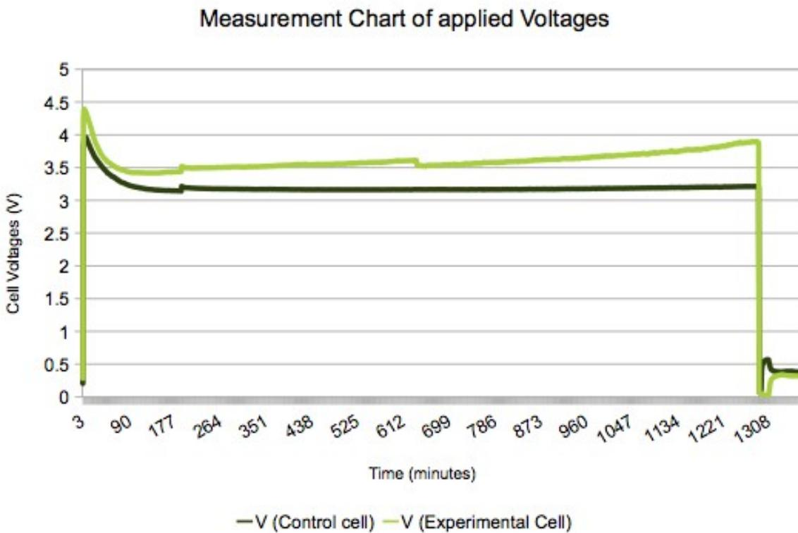
*Figure 3: Comparative measurements of temperature and voltage of the cells. We can see the adjustment of potential on the power supply and the differences of evolution of the temperatures. The current is constantly maintained to 3.5A by the power supply.*
