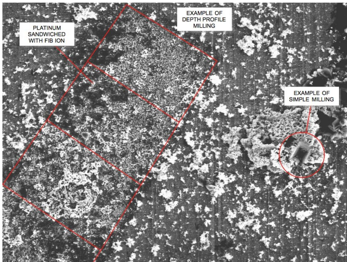
Figure 10: Example of millings made on the surface. The milling pattern is represented in red and is 50 $\mu$ m in width. A solid square is milled on a platinum stack on the right side.
