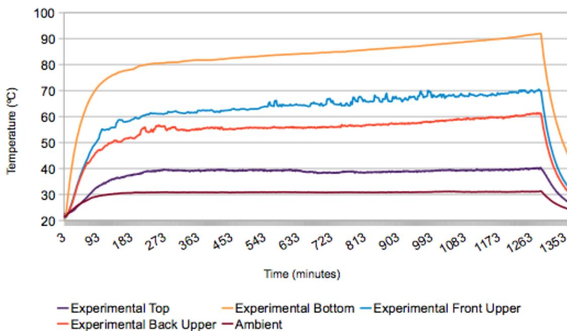
Figure 2: Temperature measurements of each cell at different locations on the cell beaker. We can see how the experimental cell temperature reached higher temperature than the control cell continuously after the first 200 minutes.
