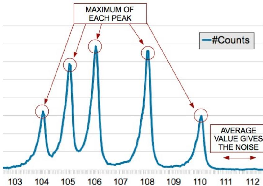
Figure 27: Example of data extraction from the measurements.
