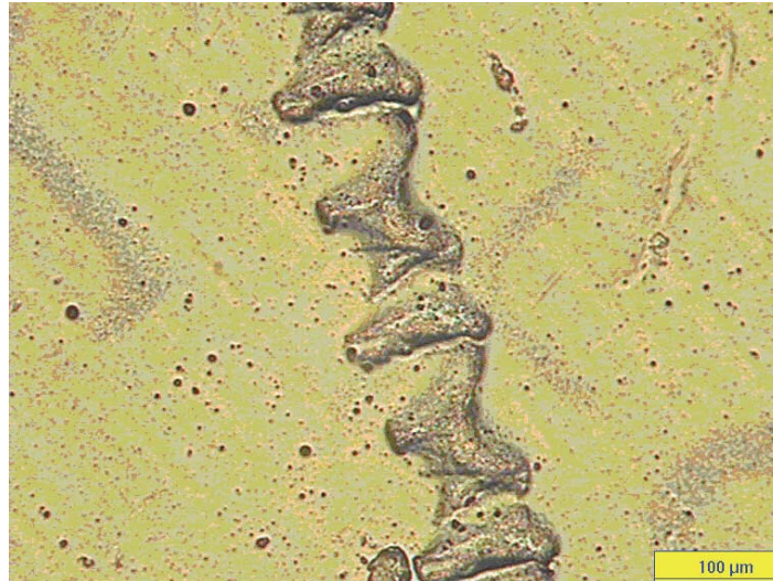
Figure 15. Residual trail mark on emulsion. It is about 100 \mu\text{m} wide. Urutskoev and Savvatimova have called patterns like these “tire-track” markings. At lower magnifications, they look like dark lines. The scale is about 100 \mu\text{m} .
