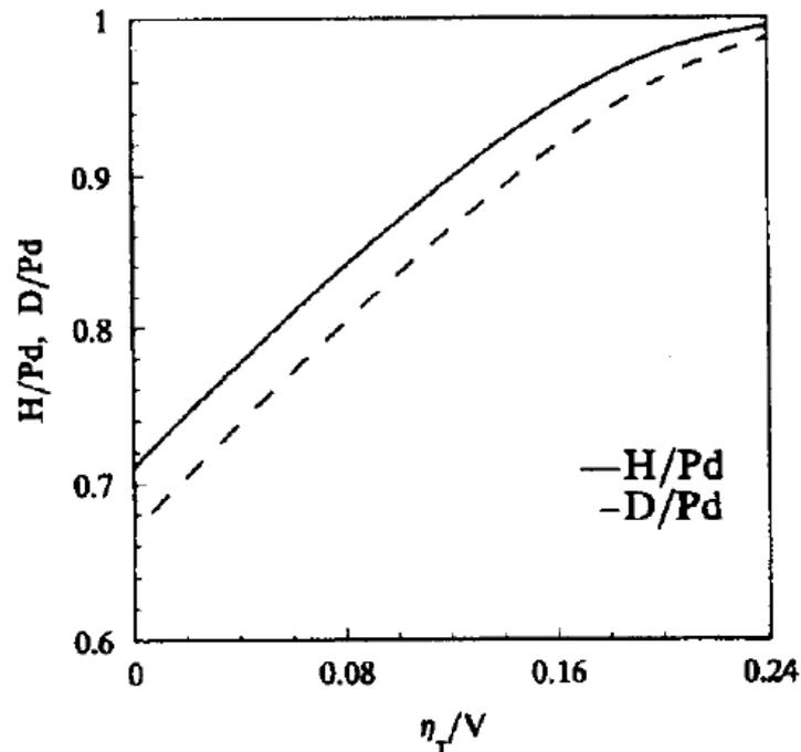
Fig. 1. Dependence of the loading ratio,  $x = H/Pd$  ( $D/Pd$ ), on  $\eta_T$ , the overpotential of the Tafel step.  $f_{H_2,0} = f_{D_2,0} = 1$  atm,  $T = 298$  K.
