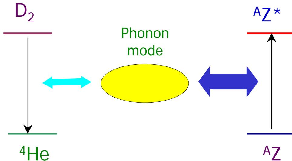
Indirect evidence from experiment implicates  $\text{AZ} = {}^4\text{He}$ , and theory and experiment suggest that  $\text{AZ}^*$  is a localized two-deuteron state
