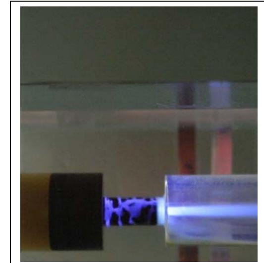
**6 STAGE.** At increasing of pressure up to 90-95 atmospheres the process of sharp increasing of intensity of this white-blue directed beam takes place. The frequency of lightnings formation is also increasing.
