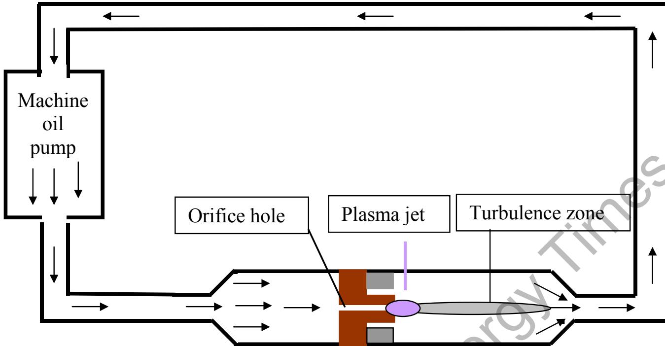
At such conditions in the volume of cavitating zone the small blue plasma jet is shaped. It forms in the region of turbulence and cavitations of circulating stream of the liquid immediately behind the orifice hole of a diaphragm. Such stationary plasma jet has the longitudinal size and diameter about 2 mm.
