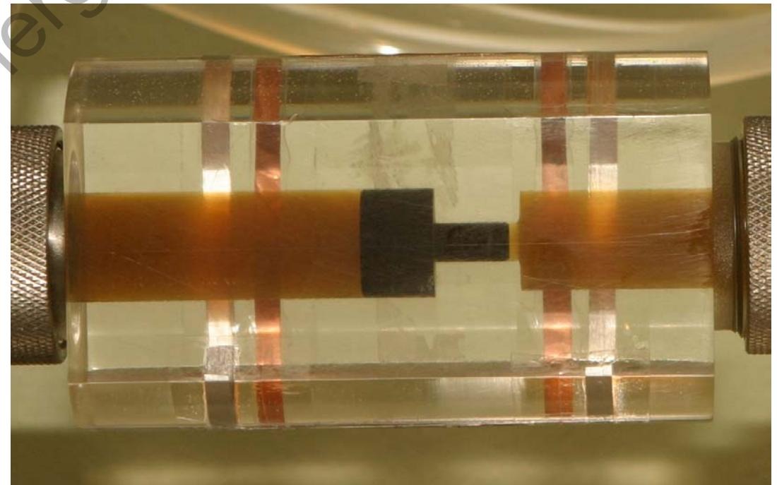
**2 STAGE** At pressure about 30 atmospheres the process of formation of cavitation bubbles in the volume behind the orifice hole starts. In this area at such pressure the process of initial turbulence and generation of large size fluctuations of machine oil density behind the orifice hole takes place. These fluctuations are visible.
