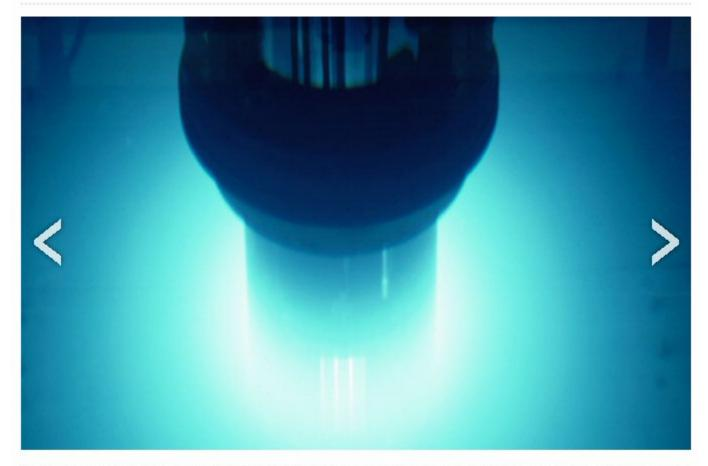
A water-cooled nuclear core glows blue as rock samples are irradiated to make them radioactive so that the gamma-ray spectrum can be studied. ROGER RESSMEYER/CORBIS
