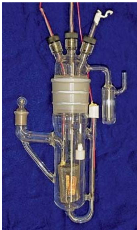
First Generation Palladium-deuterium codeposition cell was used in early cold fusion research. Courtesy of Steven B. Krivit
