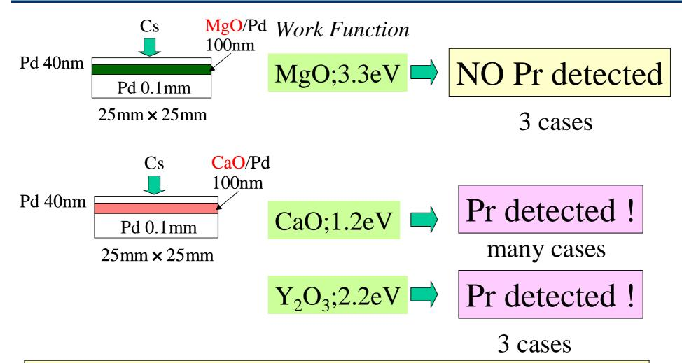
Work function of the intermediate layer is important?
