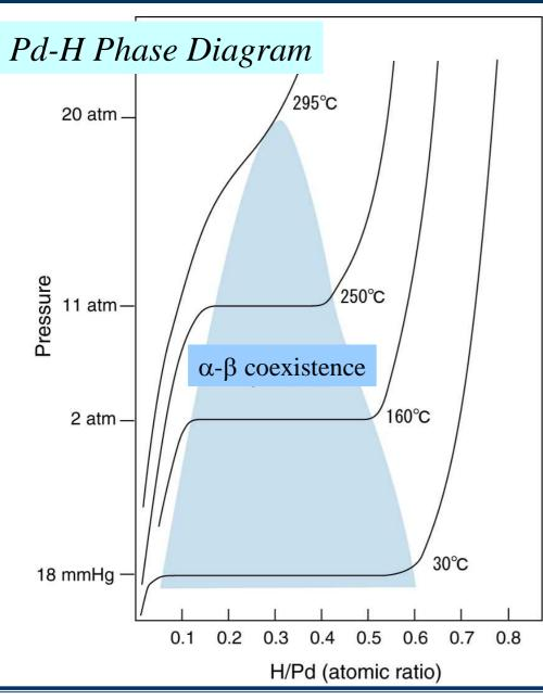
PdH<sub>x</sub> at RT  $\alpha$ -phase: x ~ 0.06  $\beta$ -phase: x ~ 0.6
