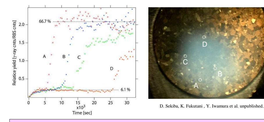
To  $\alpha$ -phase: almost simultaneously ~3,000sec To  $\beta$ -phase: Seems to be **dependent on the distance from the center**
