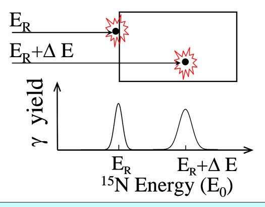
Hydrogen density distribution can be measured by 15N Ion beam
