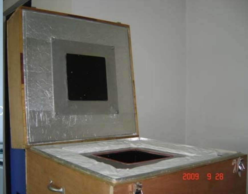
Photo of Seebeck Envelope Calorimeter (SEC)
