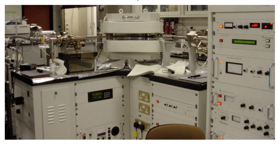
77K activated charcoal trap/metal getters for hydrogen isotopes 1400°C inlet for He absorbed in Pd
