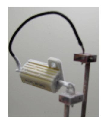
$1.008\Omega$  at 298K,  $0.988\Omega$  at 77K
