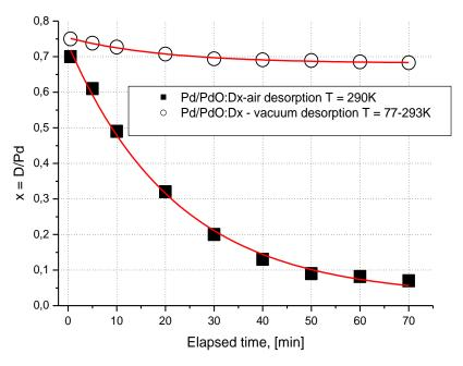
D-desorption rate from the Pd/PdO:Dx samples in vacuum (electrolysis at T=280 K with cooling down to T=77 K after electrolysis termination)) and in air at ambient conditions (electrolysis at T=290 K).
