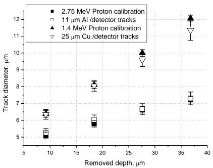
The black squares and triangles represent fit of experimental tracks from detectors 1 and 2 (empty squares and triangles, respectively) with d(h) functions obtained using normal incidence accelerator CR-39 bombardment at proton energies 2.75 (consistent with 3 MeV proton after its passage through 11  $\mu$ m thick Al foil) and 1.4 (consistent with to 3 MeV proton after its passage through the 25  $\mu$ m thick Cu foil) MeV , respectively .
