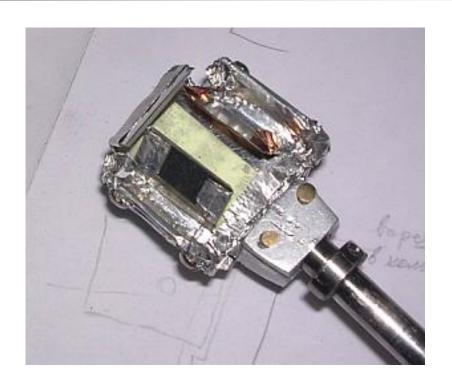
SEM with sample holder inside (left); test of the e-beam position and size (8x6 mm2) using a luminophore plate at the sample position (right).
