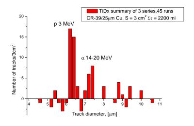
Both statistically significant 3 MeV proton (5.2-5.4  $\mu$ m track diameter) and 11-20 MeV alphas (7.0-7.6  $\mu$ m track diameter) bands are appeared in the 11  $\mu$ m Al covered detector (left); bands of 1.5 MeV protons (track diameter 6.0-6.6  $\mu$ m, consistent with the 3 MeV proton losses in 25  $\mu$ m Cu foil) and 14 MeV alphas (track diameter near 7.4  $\mu$ m, consistent with  $\sim$  17 MeV alpha losses in 25  $\mu$ m Cu foil are detected (right)
