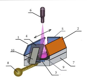
1,2 and 3 – are the CR-39 detectors covered with the 11  $\mu$ m Al (1), 25  $\mu$ m Cu (2) and 33  $\mu$ m Al (3) foils, respectively, 4 –deuterated sample, 5-manipulator, 6-electron gun, 7- stainless support
