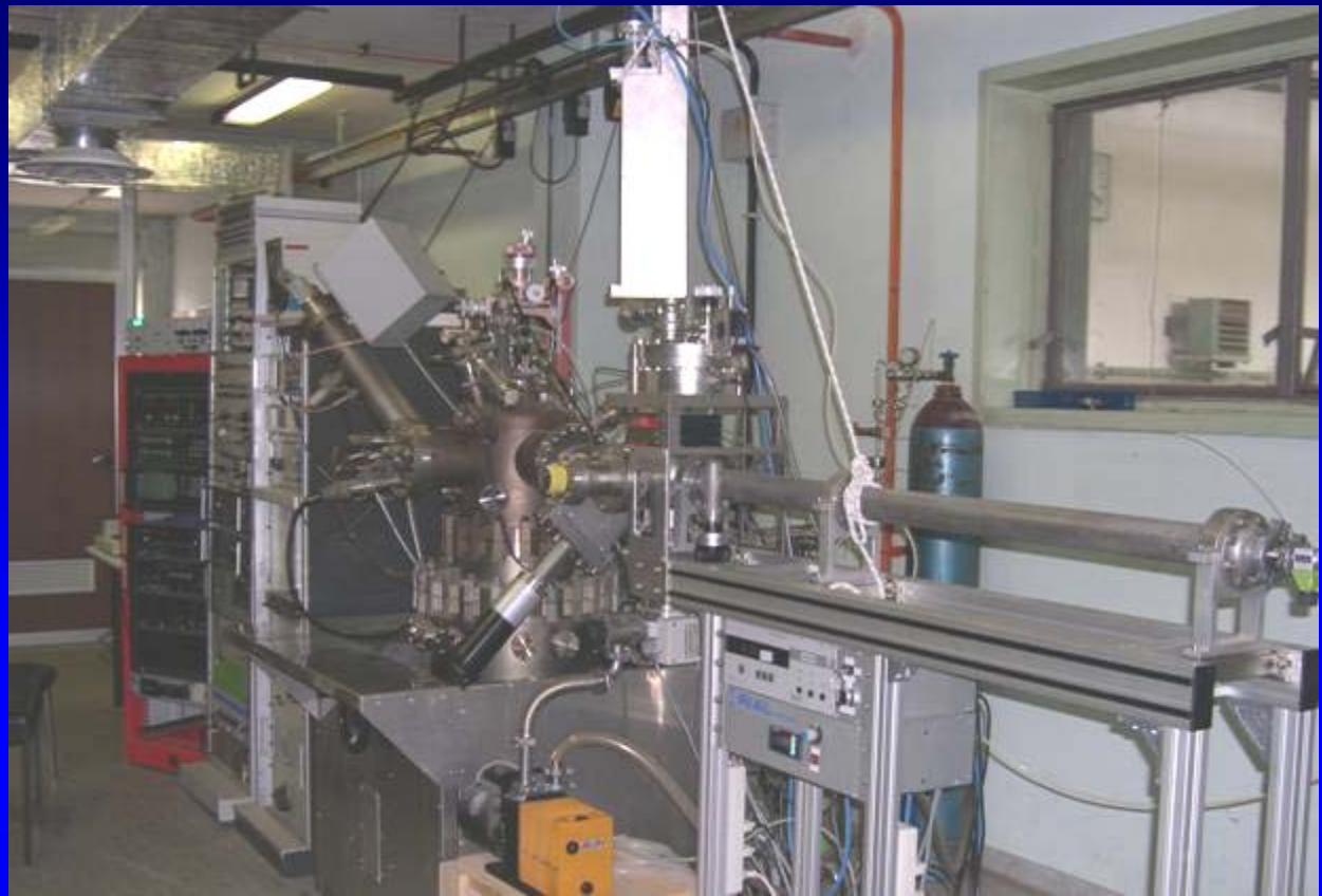
Leybold SSM200-Mass Spectrometer Module at ENEA Frascati Lab. (Italy)
