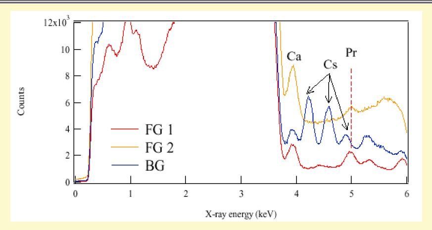
Detection of Pr using SOR X-ray at Spring-8, Harima, Japan (FG1,FG2:Signals from Samples after D2 Permeation BG:Signals from the sample before Permeation)
