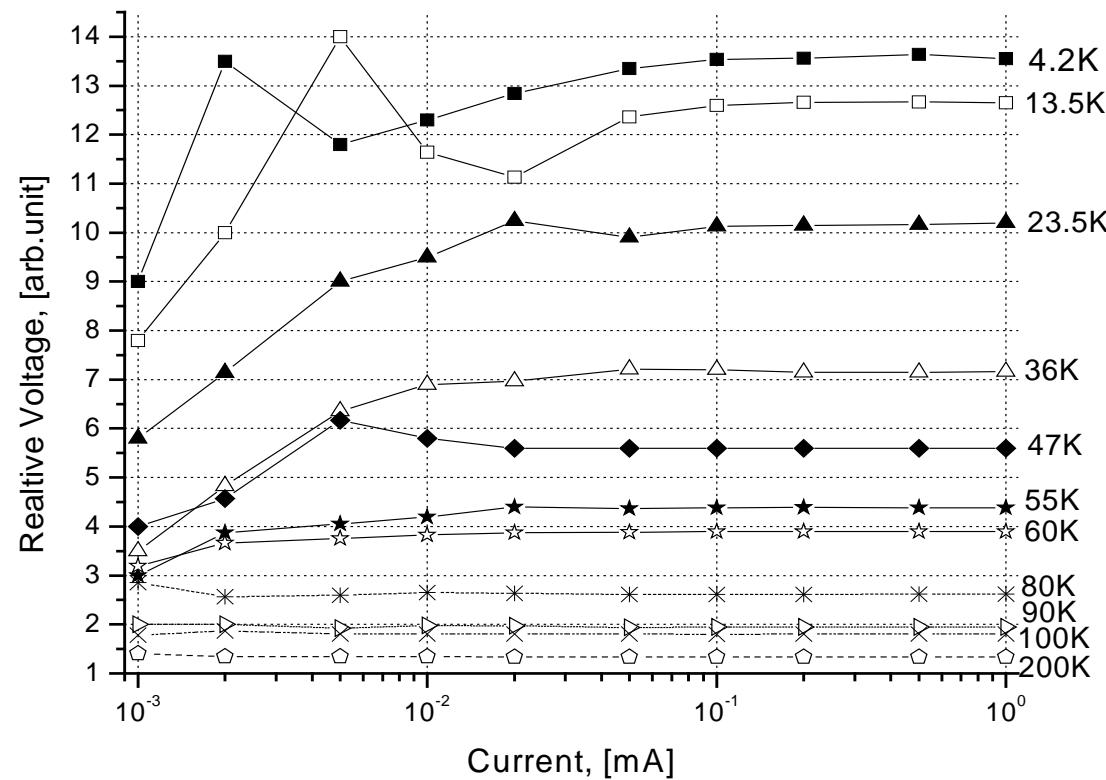
2-probe resistance measurement: Relative resistance of Pd-PdO:H<sub>x</sub> boundary [ $R(\text{Pd/PdO:H}_x)/R(\text{Pd/PdO})$ ] vs. T.
