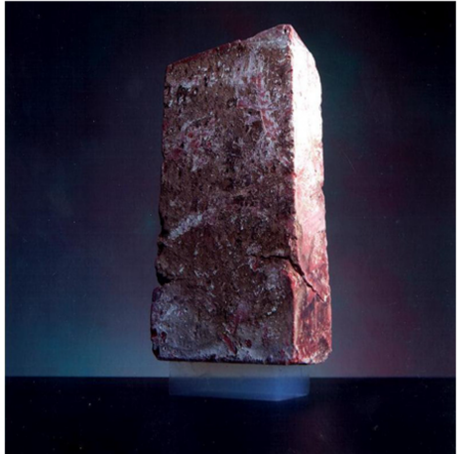
Aerogel Supporting a Brick
