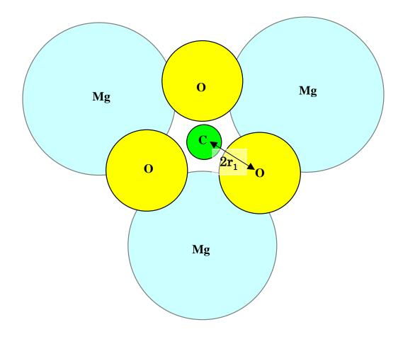
Fig.2 Configuration of  $CO_3$  group atoms in (111) magnesite crystal planes. The  $CO_3$  group lies exactly midway between the planes on which the Mg atoms lie.
