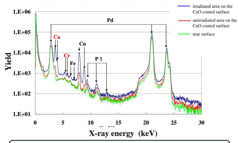
PIXE spectra for irradiated, unirradiated and rear surface of the CaO/Pd sample after 20- and 12-keV D<sup>+</sup> irradiation
