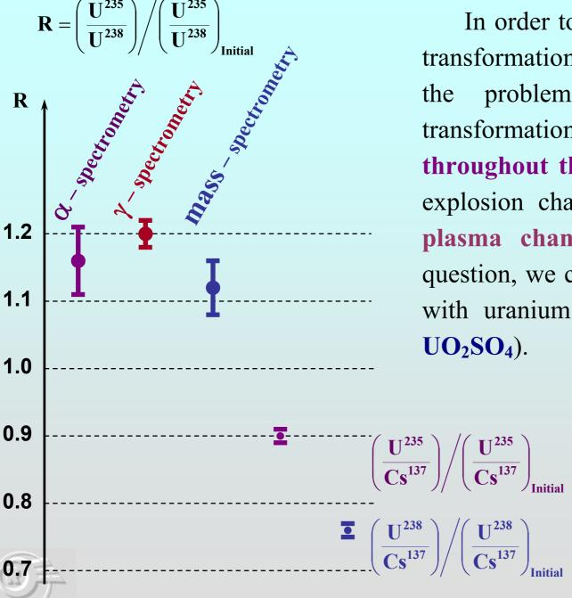
In order to complete the story of transformation, we should discuss the problem: where does transformation take place, either throughout the whole space of the explosion chamber or only in the plasma channel? To answer this question, we carried out experiments with uranium salts (uranyl sulfate,
