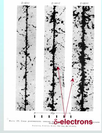
In another **Figure**, a <u>typical track</u> created by an ion in a nuclear emulsion is shown for comparison. One can readily see that the traces we have found are much broader. Moreover, they are not continuous; frequently are narrower, and traces of **5-electrons** cannot be seen at all. Such traces (hairs) are always observed when high-energy particles are absorbed.
