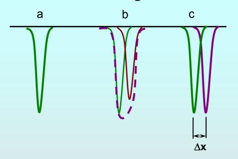
Our experimental search for the monopole started with an attempt to capture it in a ferromagnetic trap. Foil made of iron fifty seven was used as such a trap. The idea was that capture of the monopole by the ferromagnetic will change the field on the Fe<sup>57</sup>. This in turn will affect the width of Mössbauer spectrum lines.
