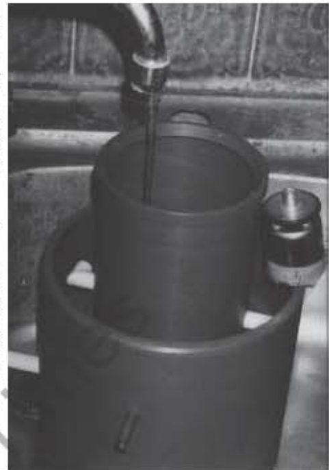
Fig. 3. Photograph of the Segner-Marinov turbine.
