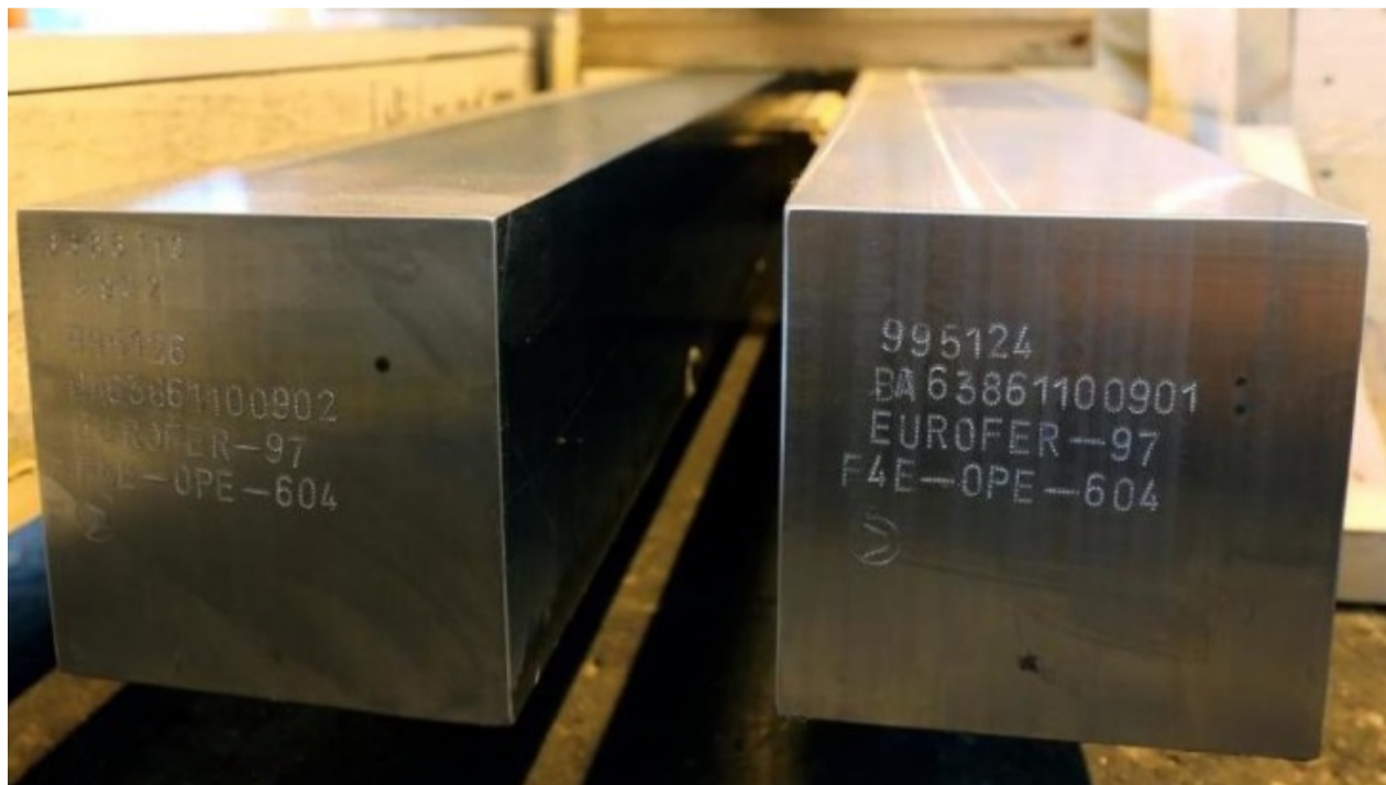
Blocks of Eurofer97 alloy steel (Image: Saarschmiede)
