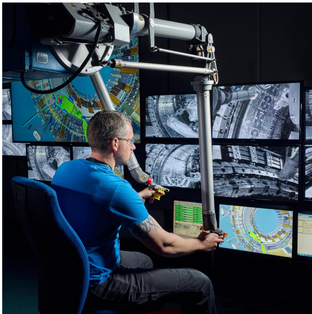
Arm's length: an operator controls robot handlers working inside Jet's reactor
