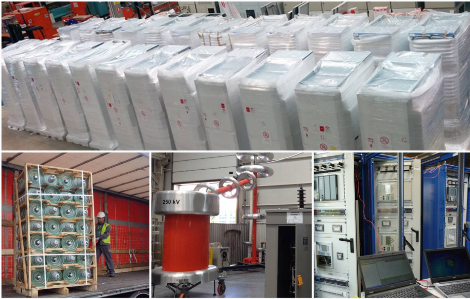
Electrical components procured by PPPL are shown clockwise: switchgear, high-voltage protection and control cubicles, resistors and insulators. Photo courtesy of © ITER Organization Photo courtesy of © ITER Organization
