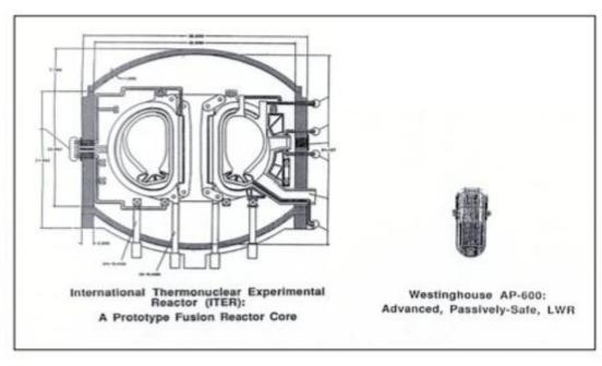
An LLNL **1994** comparison between the ITER core & the core of the comparable power Westinghouse Advanced AP-600 nuclear reactor indicated a
