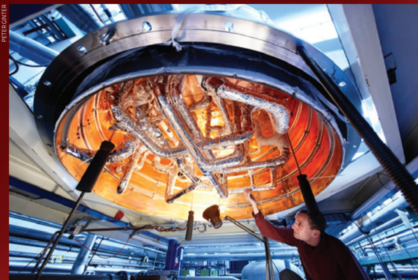
A technician in Forschungszentrum Karlsruhe, Germany, makes final checks of the prototype ITER cryogenic vacuum pumps
