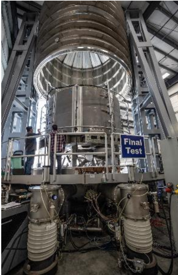
PHOTO CAPTION: Module 1 of the Central Solenoid in the final stages of testing. Courtesy General Atomics.
