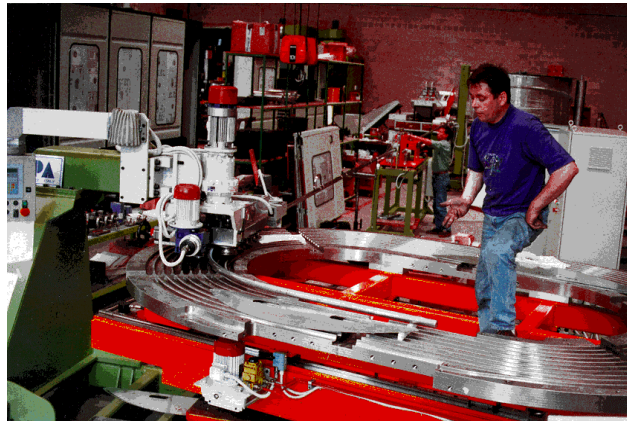
Figure 2.1.10-3 Winding TF Model Coil Conductor into Mould
