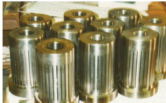
Figure 1.5.4-1 Flexible Mechanical Attachments made of Ti-Alloy (RF)
