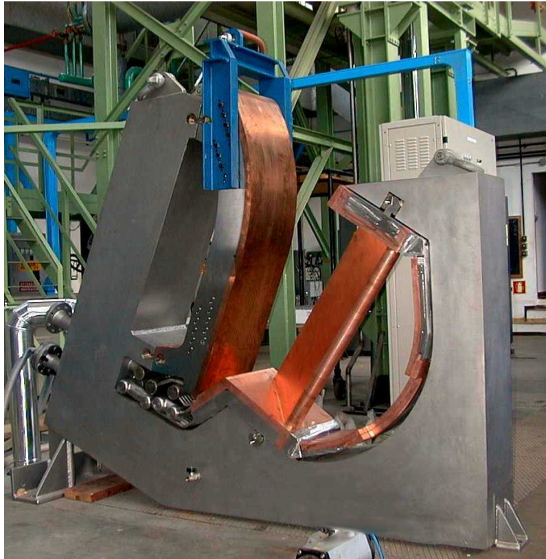
Figure 1.5.5-1 Integrated Outer Divertor Cassette (EU)
