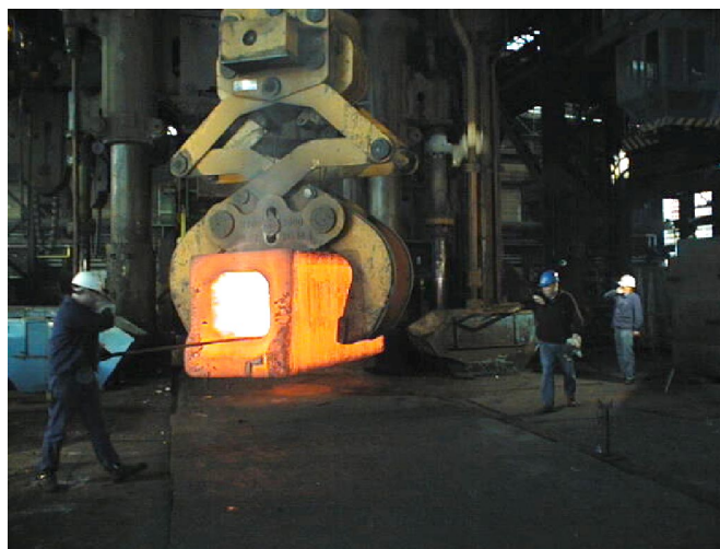
Figure 2.1.10-4 Forging of Inner Leg Curved Section of TF Coil Case as Hollow Tube
