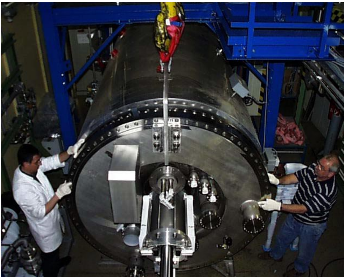
Figure 1.5.7-1 50% Scale Cryogenic Pump (EU)
