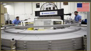
• 1,000-ton Central Solenoid fabrication on-going
