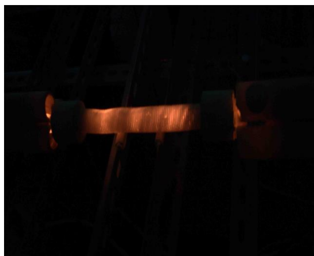
Figures 12a, 12b. E-Cat operating during the test. Note the Inconel resistors leaving the caps and entering the rods, where they are connected to the copper cables of the power supply. The resistors appear to glow intensely in the parts lying outside the caps, whereas inside the reactor body they seem to shade an underlying emission of light. This may be explained if we consider that the main source of energy inside the reactor body is actually the charge, and that it is emitting more light than the resistors. These are not visible through the caps, which are thicker than the reactor body. Upon leaving the reactor, however, the resistors emit heat almost exclusively by radiation (convection is negligible here, as they are inside the rods): there are no brighter sources of light which can “outshine” them, nor masses of alumina that can cool them. Their temperature is moreover fairly high, on account of the current they carry and the heat extracted by conduction from the reactor. Figure 12b was taken in the dark, from the opposite side to that of 12a. One of the three sets of hollow rods is visible, and another patch of insulating alumina cement on the second metal strut in the middle, added without modifying the setup.
