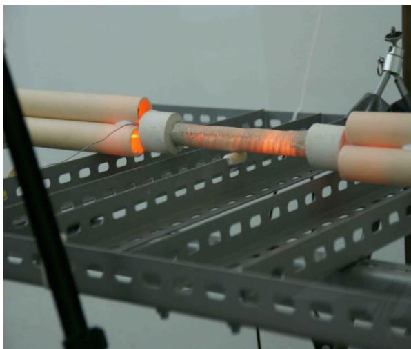
Figures 12a, 12b. E-Cat operating during the test. Note the Inconel resistors leaving the caps and entering the rods, where they are connected to the copper cables of the power supply. The resistors appear to glow intensely in the parts lying outside the caps, whereas inside the reactor body they seem to shade an underlying emission of light. This may be explained if we consider that the main source of energy inside the reactor body is actually the charge, and that it is emitting more light than the resistors. These are not visible through the caps, which are thicker than the reactor body. Upon leaving the reactor, however, the resistors emit heat almost exclusively by radiation (convection is negligible here, as they are inside the rods): there are no brighter sources of light which can “outshine” them, nor masses of alumina that can cool them. Their temperature is moreover fairly high, on account of the current they carry and the heat extracted by conduction from the reactor. Figure 12b was taken in the dark, from the opposite side to that of 12a. One of the three sets of hollow rods is visible, and another patch of insulating alumina cement on the second metal strut in the middle, added without modifying the setup.
