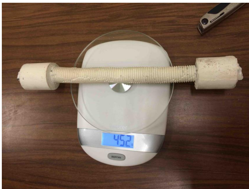
Figure 1. Weighing the E-Cat after the test (452 g). The ridges along the body of the reactor increase the dissipation surface for natural heat convection. The power supply cables run through the two cylindrical extremities (termed "caps"), and were cut prior to weighing.
