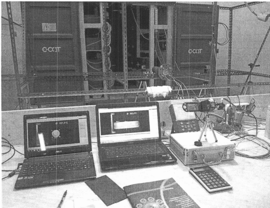
Fig. 11. Instrument set-up for the test. From left to right: the two laptops connected to the IR cameras, framing the “top” (i.e. the base) of the E-Cat HT2 and one of its sides, respectively, plus the video camera, and the PCE-830. Background: the E-Cat HT2 resting on metal struts and the two IR cameras on tripods.
