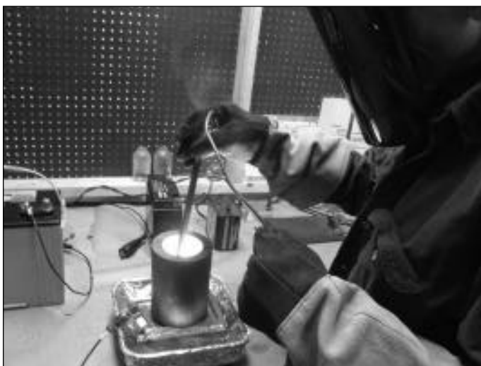
Charging graphite powder with graphite rod and crucible.
