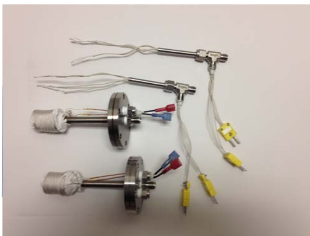
Figure 3.5 Design and photographs of the welded cell configuration and the thermocouple inserts.
