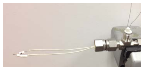
Figure 3.2 Custom feedthrough and thermocouple used for interior cell temperature measurements.
