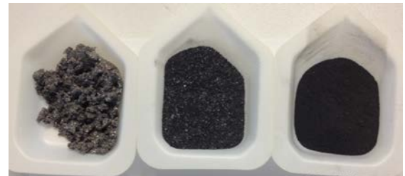
Figure 2.2. ZrO 2 NiPd after ground with a mortar & pestle (center) and 4 minutes in power grinder (right). The left sample is the SmCo magnetic after it was ground with a mortar & pestle
