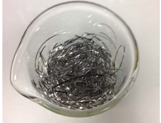
Figure 2.1. Approximately 10 grams of 65wt% Zr- 32wt% Ni-3wt% Pd alloy melt spun ribbon in a 1L breaker used for furnace oxidation.
