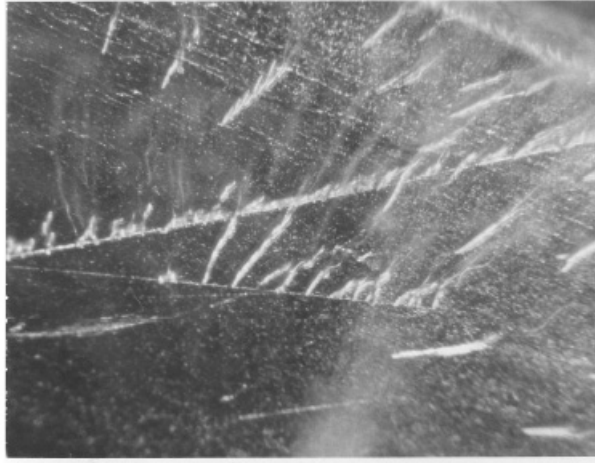
Figure 4. Bubbles of D 2 arising through acetone from cracks in PdD after electrolysis. The bright lines at which bubbles are forming are surface scratches that focused formation of a deeper crack structure.
