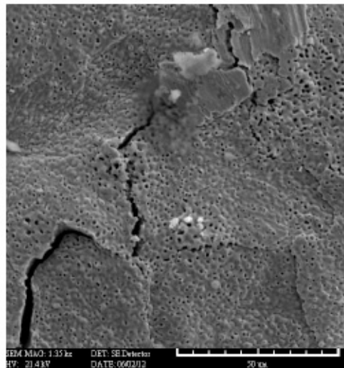
Figure 8. SEM image of a surface of Ni on Pd after the study containing voids and cracks.
