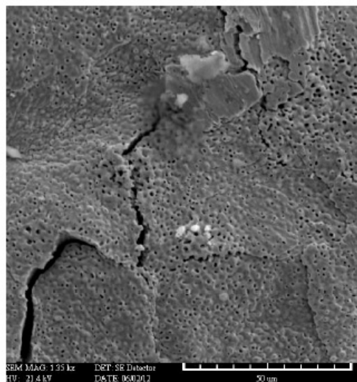
Figure 2. SEM image of a surface of Ni plated on Pd on which voids and cracks have formed.
