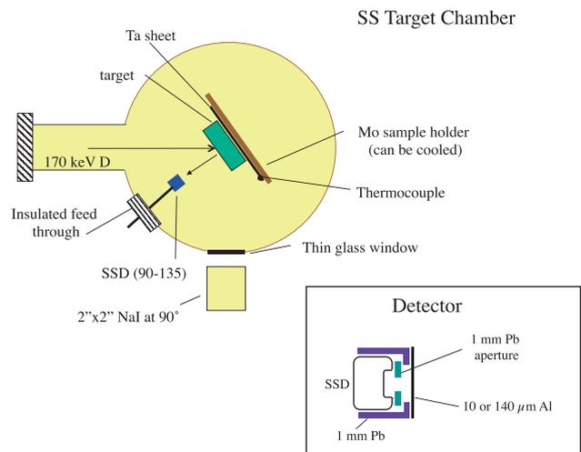
**Fig. 1.** (Color) Schematic diagram of the scattering chamber and detector configurations.
