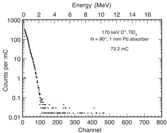
**Fig. 5.** Energy spectrum of charged particles emitted at an angle of  $90^\circ$  from a  $\text{TiD}_2$  target bombarded by 170 keV deuterium ions. A 1-mm-thick Pb foil placed in front of the detector stops protons with energy  $<20$  MeV. Paraffin shielding was removed from around chamber.
