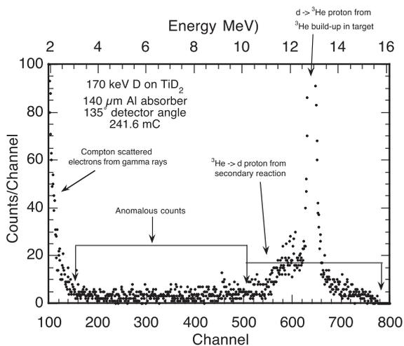
**Fig. 8.** Energy spectrum of charged particles emitted at an angle of  $135^\circ$  from a  $\text{TiD}_2$  target bombarded by 170 keV deuterium ions. A  $140\text{ }\mu\text{m}$  thick Al foil was placed in front of the detector.
