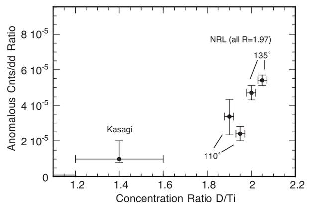
**Fig. 10.** The ratio of yield of anomalous counts to the yield of 3 MeV protons from the (p, t) branch of the d–d reaction versus the D/Ti ratio of the target. The data point at D/Ti of 1.4 is from ref. 1. The four data points at D/Ti = 1.97 are from this work.
