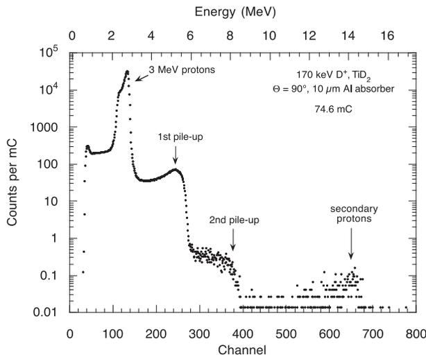
**Fig. 2.** Energy spectrum of charged particles emitted at an angle of  $90^\circ$  from a  $\text{TiD}_2$  target bombarded by 170 keV deuterium ions. A 10- $\mu\text{m}$ -thick Al foil in front of the detector stops elastically scattered deuterium.
