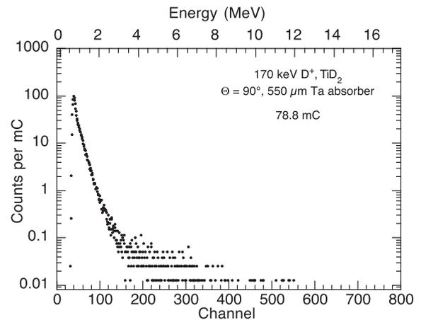
**Fig. 4.** Energy spectrum of charged particles emitted at an angle of  $90^\circ$  from a  $\text{TiD}_2$  target bombarded by 170 keV deuterium ions. A 550- $\mu\text{m}$ -thick Ta foil placed in front of the detector stops protons with energy  $<20$  MeV. Paraffin shielding was placed around the chamber.
