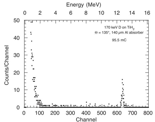
Fig. 7. Energy spectrum of charged particles emitted at an angle of  $135^\circ$  from a  $\text{TiH}_2$  target bombarded by 170 keV deuterium ions. A  $140\ \mu\text{m}$  thick Al foil was placed in front of the detector.
