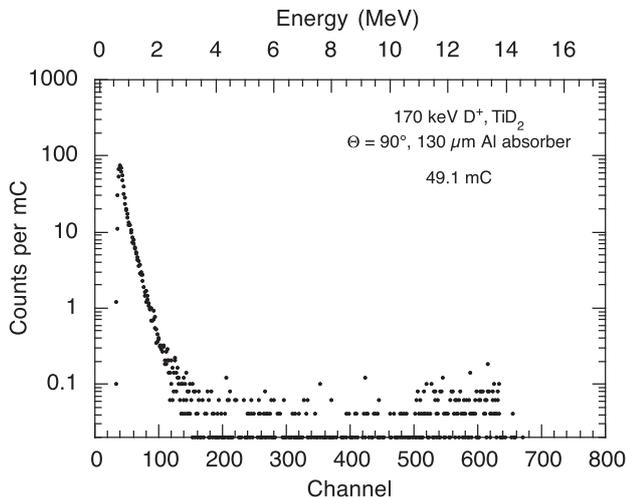
**Fig. 3.** Energy spectrum of charged particles emitted at an angle of  $90^\circ$  from a  $\text{TiD}_2$  target bombarded by 170 keV deuterium ions. A 130- $\mu\text{m}$ -thick Al foil in front of the detector stops protons with energy  $<4$  MeV.
