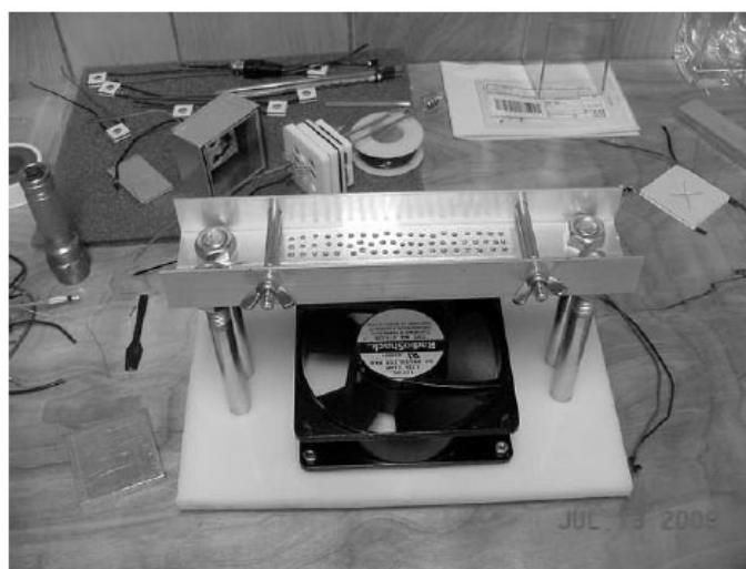
Figure 5. A rack was constructed from commonly available parts; the aluminum trough was perforated to allow uniform air flow over the heat sinks. Two thermistors were placed in the aluminum trough to provide precise control of the air temperature as it flows over the heat sinks.
