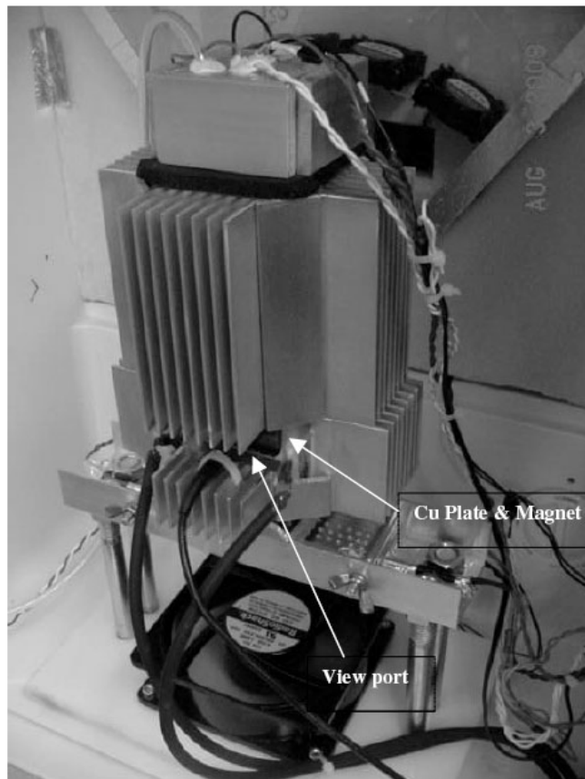
Figure 1. The Seebeck Cell Calorimeter is shown inside a temperature controlled enclosure on top of a rack with a fan to provide vigorous air stirring and a consistent airflow over the heat sinks attached to the TECs and the cell walls. Airflow temperature is controlled to \pm 0.02^\circ\text{C} , stability is \pm 0.01 W.
