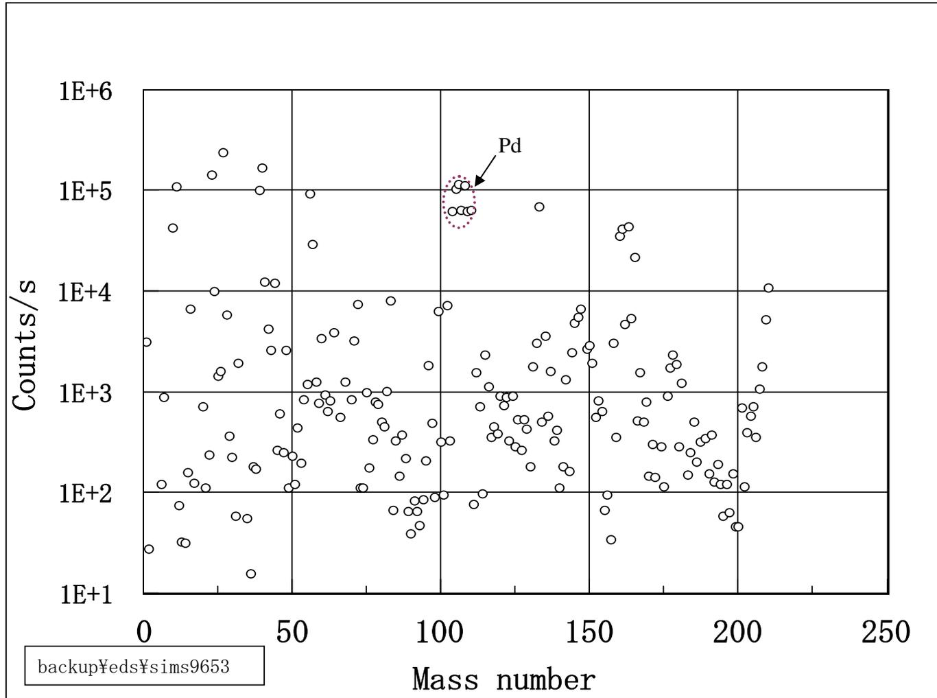
*This graph shows the mass spectrum of SIMS measurement for the Pd sample surface (1 micro meter thickness) not generated any excess heat by electrolysis. It seems rather simple compared by the before case that the Pd generated excess heat. Most different point with the excess heat is there were no Xenon, Cr, Fe, Zn and Cu.*
