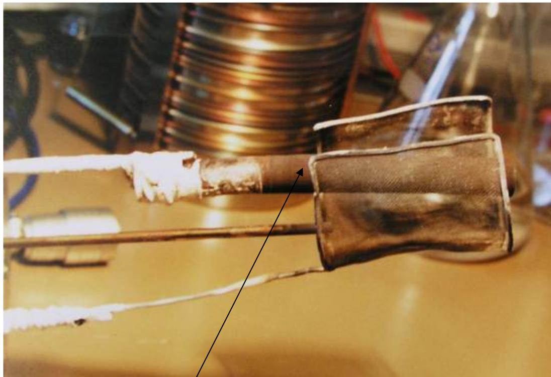
*Many elements were deposited on the electrode surface in an irregular distribution. The concentrations varied depending on the parameters of the electrolysis. The elements that have been detected on the samples were Ca, Ti, Cr, Fe, Ni, Cu, Zn, Pb and so on. The amount of each element varied by the sample lots. This may mean that some factors such as surface conditions play an important role in the reaction.*
