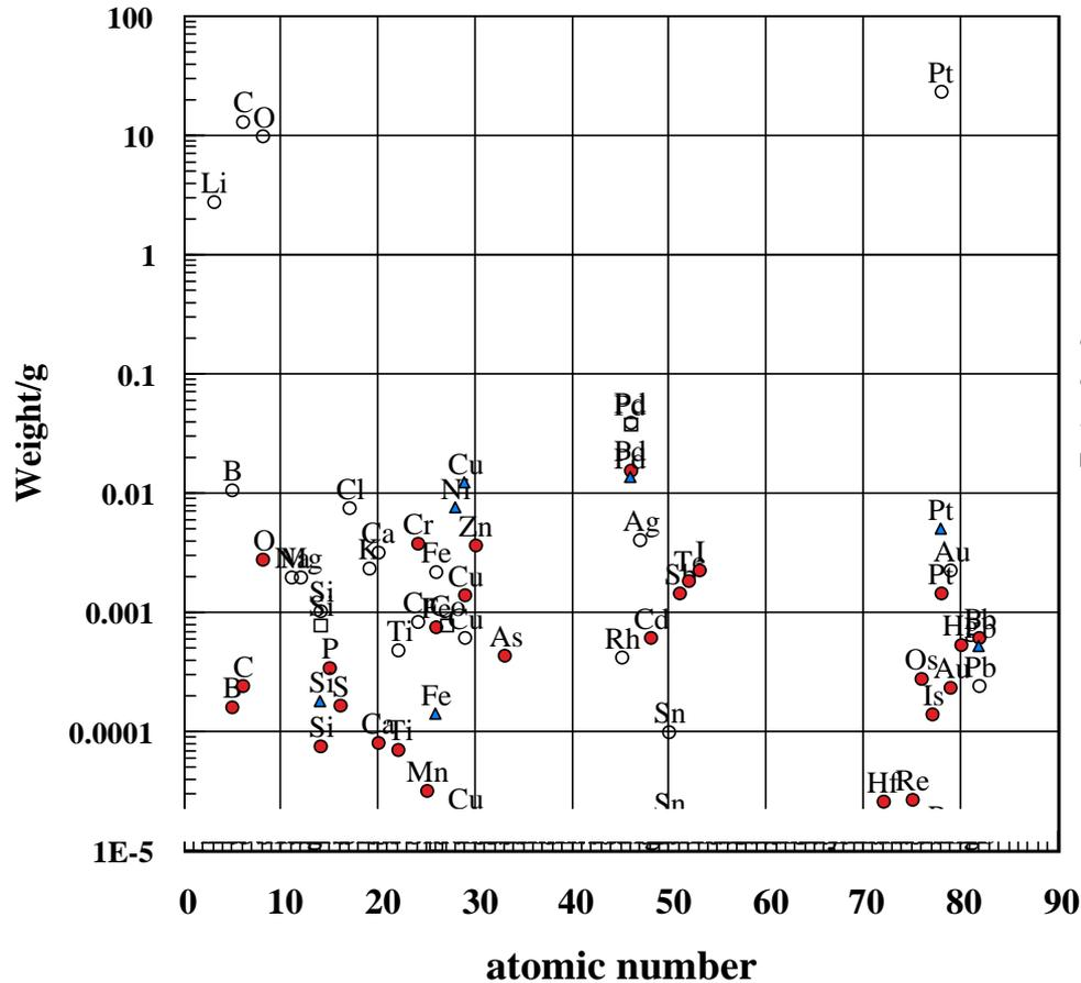
(A, ○): Sample of the before electrolysis, this includes **the solute, anode material and total impurity** in Pd, Pt and electrolyte in the cell.
