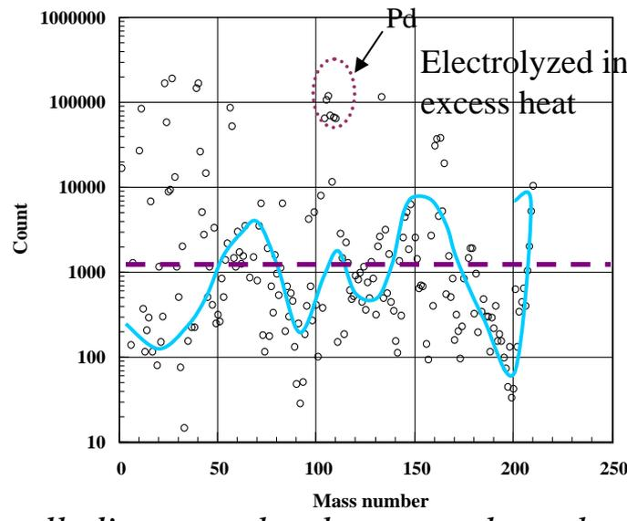
*These figures show the SIMS count spectra for palladium samples that were electrolyzed under various conditions. It is very interesting to note the change in the elements according to the electrolysis condition. The change in the elements distribution before and after electrolysis is shown as a ratio of the mass spectra.*
