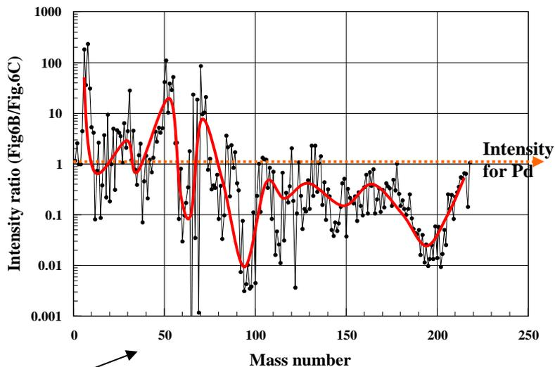
A: Intensity ratios for mass spectra for electrolysis in *heavy water with excess heat* compared to results with *no excess heat*.
