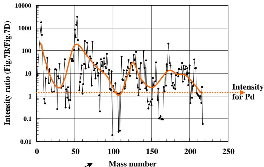
B: Intensity ratio of mass spectra between palladium in *heavy water that produced excess heat* and in *light water that produced no excess heat*.
