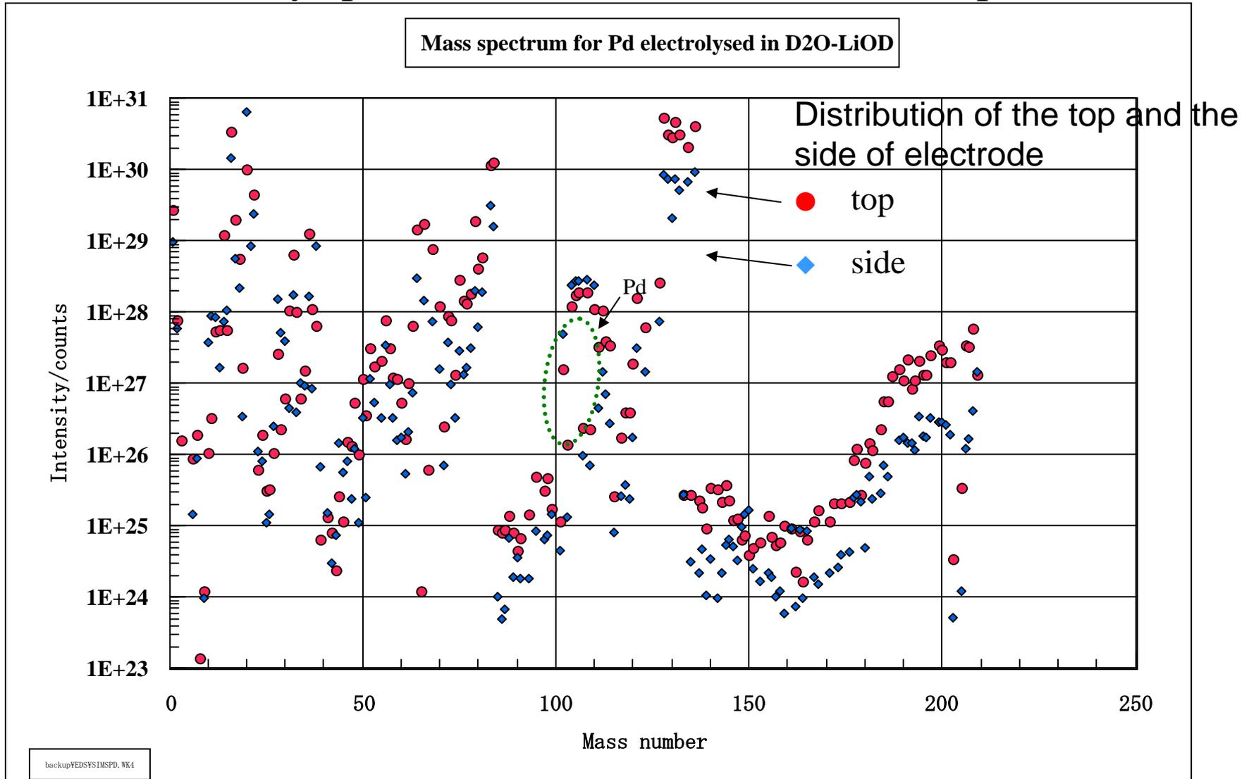
This graph shows the mass spectrum of SIMS measurement for the Pd sample surface (1 micro meter thickness) generated excess heat after electrolysis. Two of area for the sample surface were analyzed and you can see these spectra are similar. Here, the mass concentration is normalized by all AIMS count number. The spectrum has very characteristic element of Xenon. This is the inert gas and not proper element but the intensity existence is very high in the Pd electrode.
