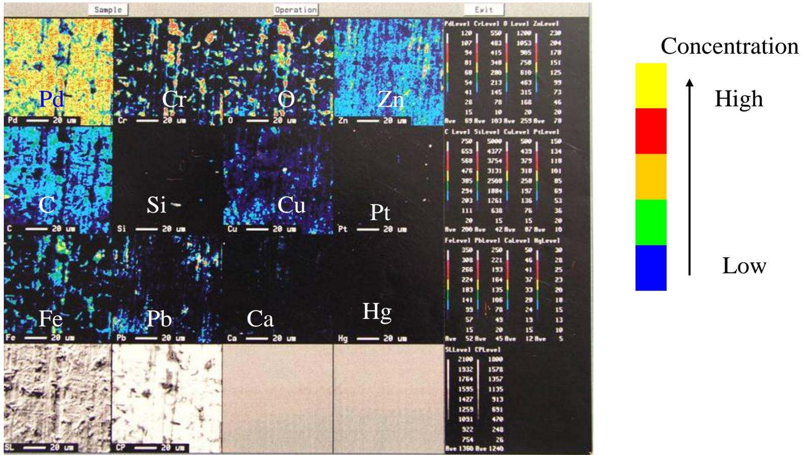
*This photo shows the element mapping for the Pd surface after electrolysis by the EPMA measurement. We can see typical deposition of Cr, Zn, Cu, Fe, Pb and others. The concentration for the elements is shown by the color that changes from white to blue. Especially, in the case, strong existence of Cr, Zn and Fe are very clear.*
