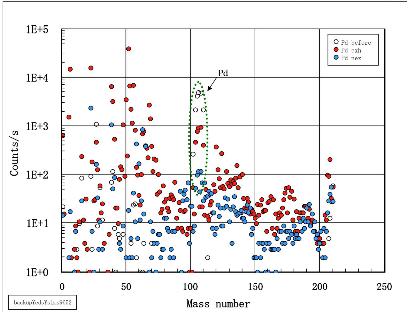
*This graph shows the mass spectrum of SIMS count for the Pd sample surface (1 micro meter thickness) before and after generated excess heat and no excess heat after electrolysis. These spectra are very different from each others.*
