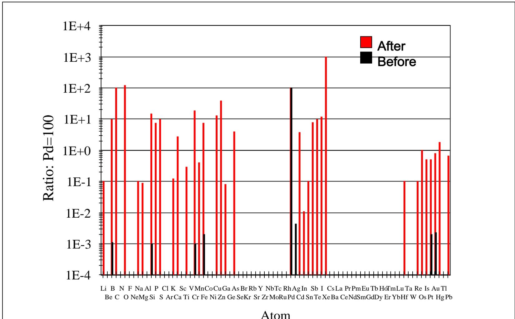
*This figure shows the relative concentration for the elements before and the after electrolysis (1 micro meter thickness). In the case, the Pd electrode generated some excess heat. The concentration for the element other than the Pd were five or six order smaller than that of Pd. However, these element increased almost same as the Pd for Cr, Zn, Xe and Cu.*
