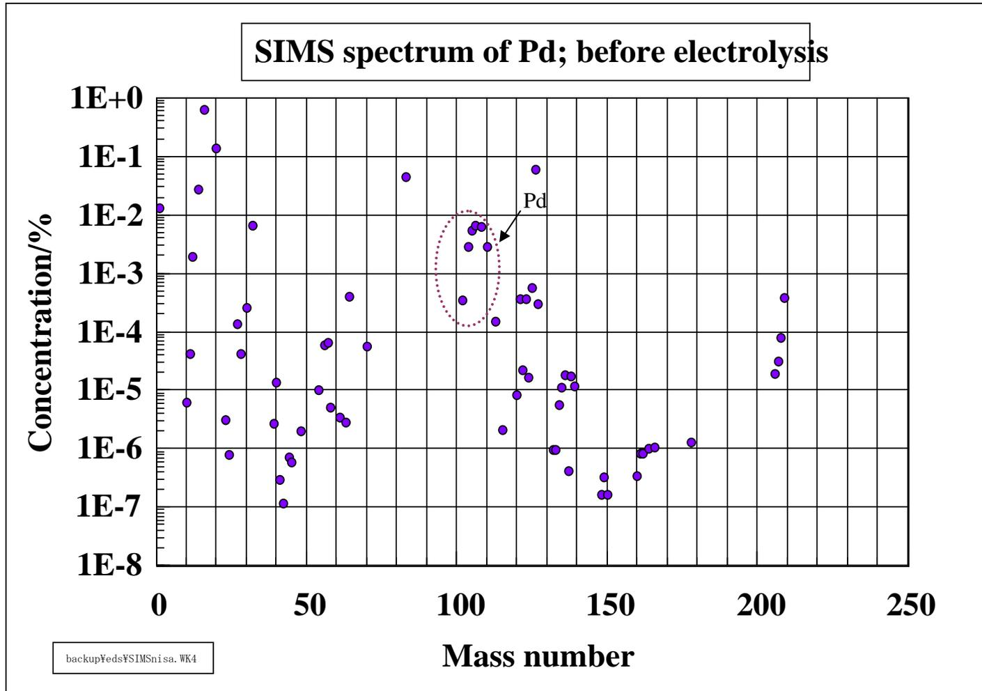
*This graph shows the mass spectrum of SIMS measurement for the Pd sample surface (1 micro meter thickness) before electrolysis. Here, the mass concentration is normalized by all AIMS count number.*
