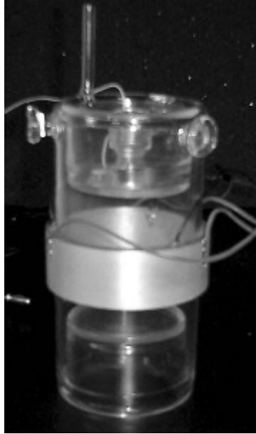
Fig. 20. Example of high-Q resonance acoustic chamber design developed by Rensselaer Polytechnic Institute (Image courtesy Richard T. Lahey).
