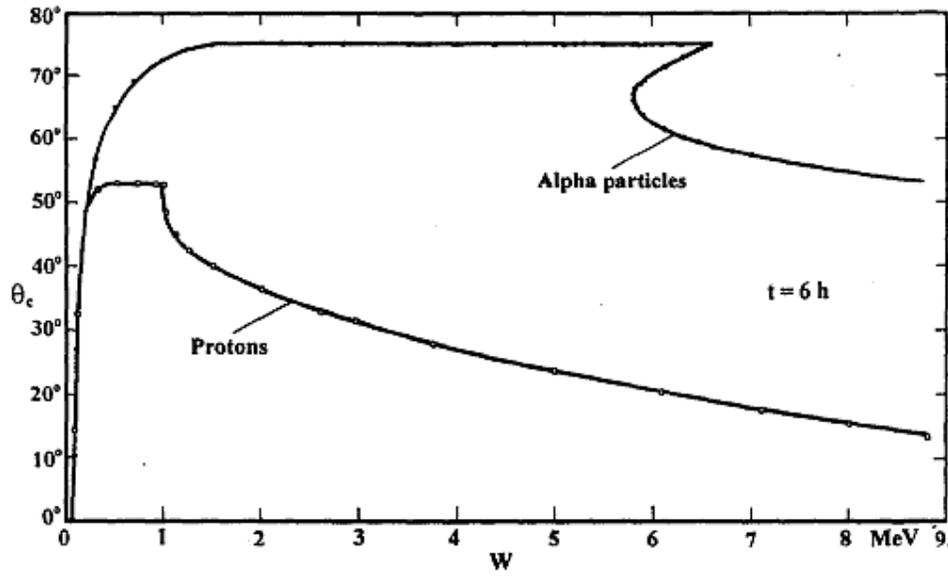
Fig. 4. Critical angle,  $\theta_c$ , as a function of the initial particle energy,  $W$ , at an etching time of  $t = 6$  h for protons and alpha particle.
