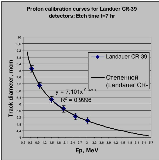
**Figure 3a** Van DeGraaf accelerator calibration curve for the 0.65-3.0 MeV proton beam of normal incidence with respect to the detector surface. The targets are Landauer RadTrack and another Fukuvi –type CR-39 detectors. Etching conditions 6N-NaOH,  $t = 70\text{ }^{\circ}\text{C}$ , for 7 hr.
