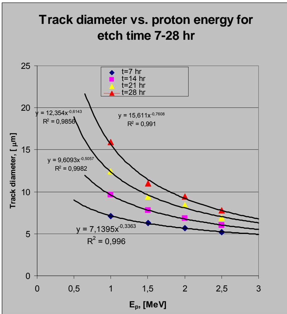
Figure 3. Track diameter vs. proton energy ( $E > 0.5$  MeV) dependences for etch time 7-28 hr.
