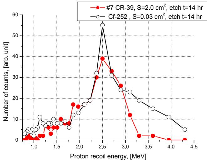
**Figure 1.** Rough reconstruction of the protons recoil spectra for CR-39 Landauer detectors obtained during electrolysis run (detector #7) and during exposure with Cf-252 neutron source. Etch time is  $t = 14$  hr. The reconstruction of the spectra was deduced from the track density vs. track diameter histograms, taking into account two functions: (a) track diameter vs. proton energies at  $t = 14$  hr, (Fig. 3) and (b) the critical angle  $\theta_c$  vs. proton energy (Fig.4).
