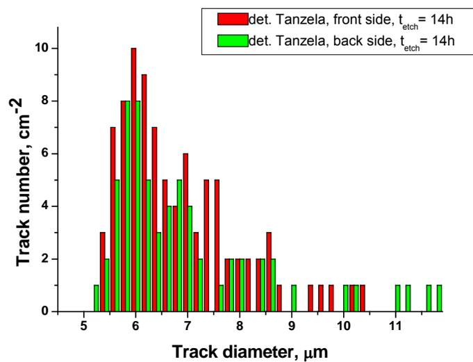
**Figure 8** Track number distribution vs. track diameter for Fran Tanzella’s # 7 CR-39 detector from both front and back sides. Etching time is 14 hr. The spectra contain real nuclear tracks.
