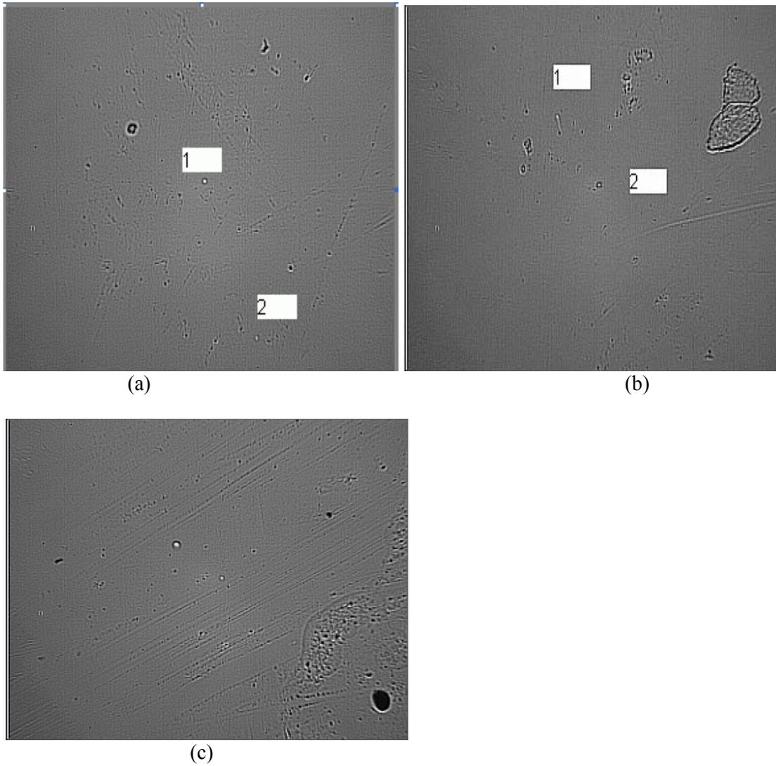
**Figure 5.** Examples of proton recoil tracks (compare with Cf-252 bright pits) of 5-7  $\mu\text{m}$  diameter from CR-39 Foreground detector #7 (removed depth is  $h \approx 8.6 \mu\text{m}$ ), images size is  $S=120 \times 90 \mu\text{m}^2$ : (a) - two tracks of normal incidence (1,2); (b) – track of oblique incidence (1), track of normal incidence (2);(c)- two tracks of normal incidence (bright pits in the center of the image).
