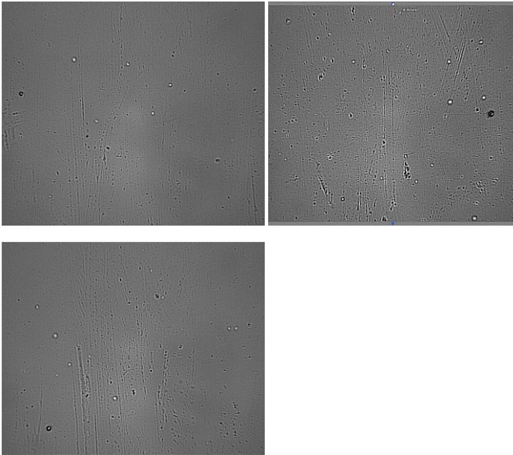
**Figure 4.** Examples of proton recoil tracks of 5-8  $\mu\text{m}$  diameter (bright pits only - all others are the surface defects !!!) for Cf-252 neutron source (7 hr etch, removed depth is  $h = 9.2 \mu\text{m}$ ): Total neutron fluence is  $F_n = 7 \times 10^8 \text{ n/cm}^2$ ; images size is  $S = 120 \times 90 \mu\text{m}^2$ .
