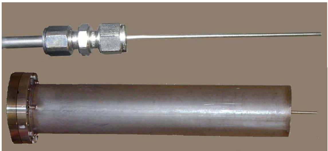
Figure 2 Top: photograph of the palladium tube attached to the stainless steel tube with a Swagelok® fitting. Bottom: photograph of the vacuum chamber
