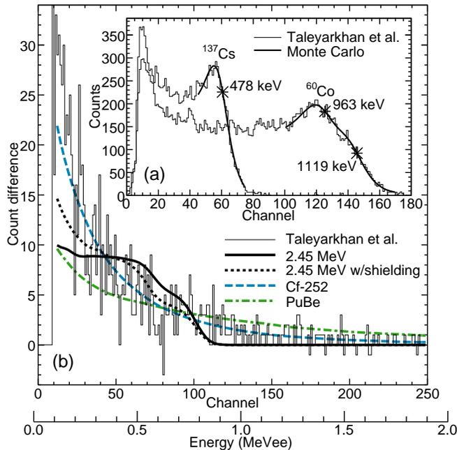
FIG. 1: (color online) Analysis of Taleyarkhan and coworkers’ liquid scintillator data. (a) Fitting the measured Compton edges of  $\gamma$  calibration sources to simulated electron recoil spectra determines the detector’s energy scale and resolution. (b) Simulated proton recoil spectra of various candidate neutron sources shown fit to data.
