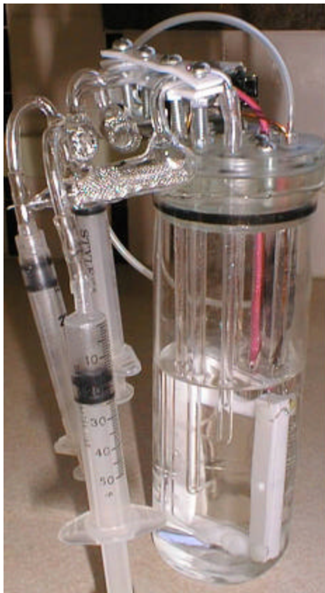
Exhibit 1b. Electrolytic cold fusion cell, approximately 14cm tall (Photo courtesy of Edmund Storms)
