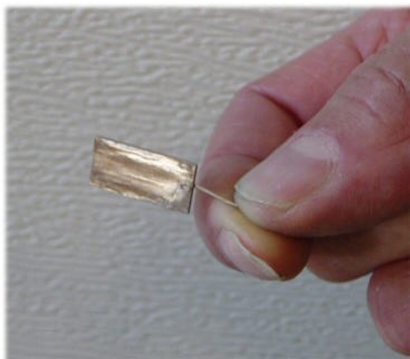
Exhibit 2. Palladium Cathode used in an Electrolytic Cold Fusion Cell (Photo by Steven Krivit)
