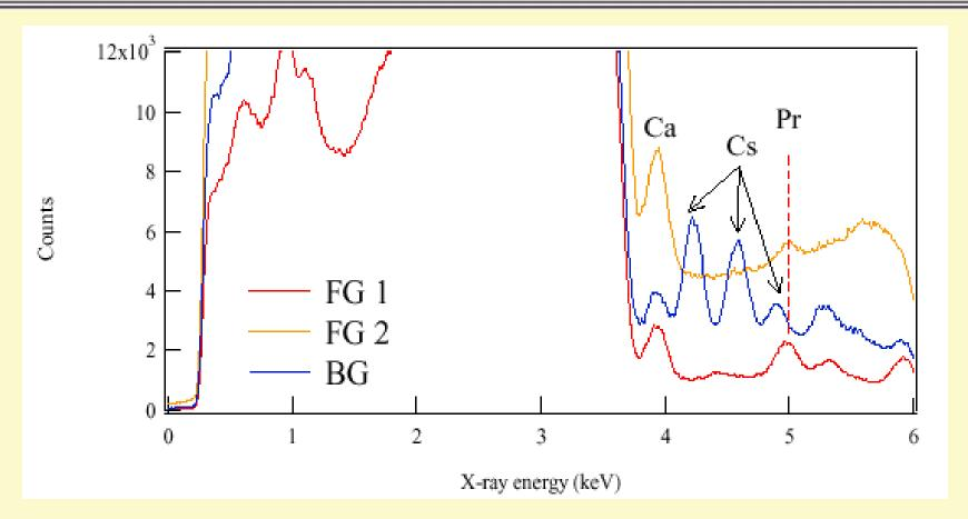
Detection of Pr using SOR X-ray at Spring-8, Harima, Japan (FG1,FG2:Signals from Samples after D2 Permeation BG:Signals from the sample before Permeation)
