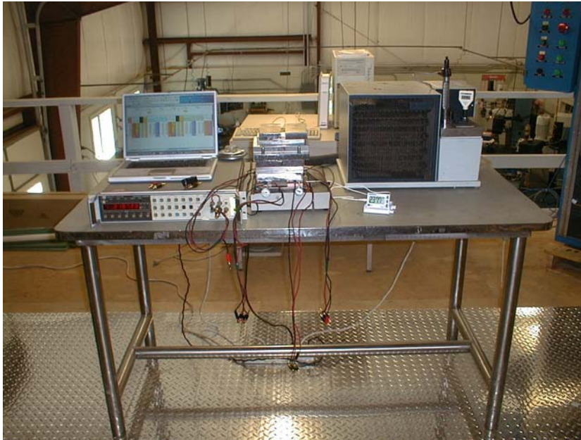
Figure D3. LTI TE wafer test apparatus.
