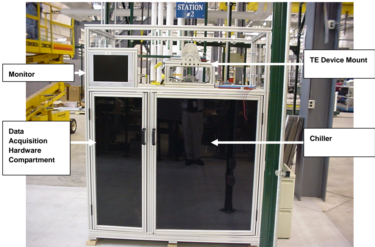
Figure 10. Thermoelectric single device test stand.
