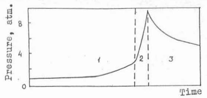
Fig.2. Working liquid pressure during switch-on (1-2) and switch-off (3) periods of the "Yusmar" hydrofacility
