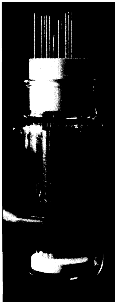
A model of the cold fusion cell that Pons and Fleischmann showed the press in March 1989.
